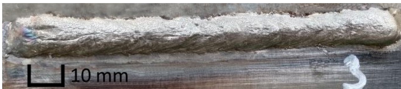
Fig. 16. External appearance of the welding bead produced by double-arc surfacing in the following mode: V_{f/w} Al=3 m/min; V_{f/w} Fe=3 m/min; V_s=0.15 m/min; U_{arc} Al=17 V; U_{arc} Fe=27.5 V
