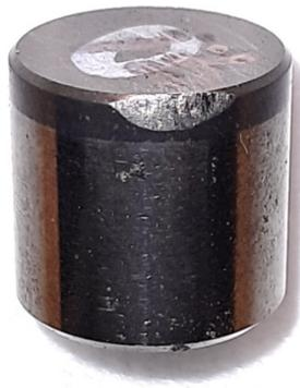
**Fig. 7.** View of the worn surface of a polycrystalline diamond insert
