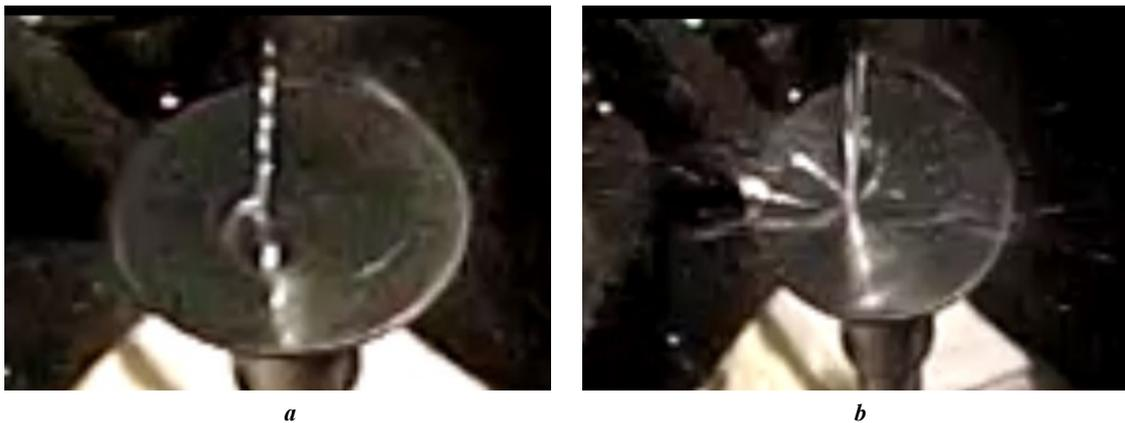
**Fig. 10.** Changing the pressure of the liquid supplied to the rough bowl surface: *a* – 1 atm.; *b* – 2 atm.
