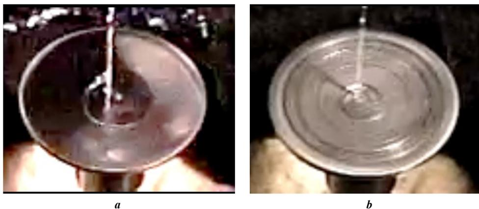
**Fig. 3.** Changing the surface roughness at a flow rate of 6.69 kg/h and a distance to the bowl of 50 mm:
