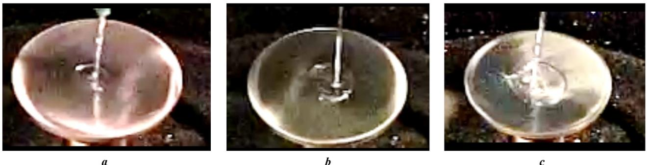
**Fig. 2.** Changing the height of liquid feed from the bowl at a flow rate of 6.69  $\text{kg/h}$  and smooth bowl processing:
