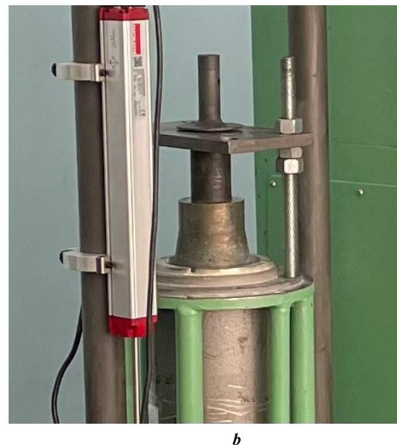
**Fig. 1.** Schematic (a) and external appearance (b) of the acoustic unit of the ultrasonic assisted ECAP device
