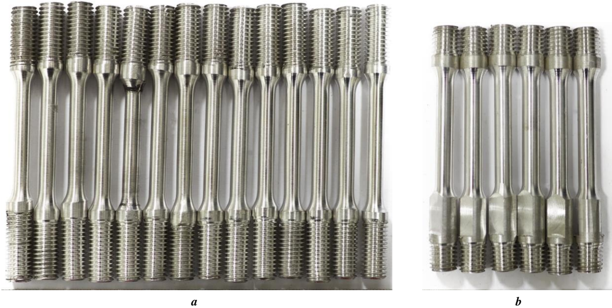
Fig. 1. Specimens for mechanical tests: a – for mass temperature-speed tests;
