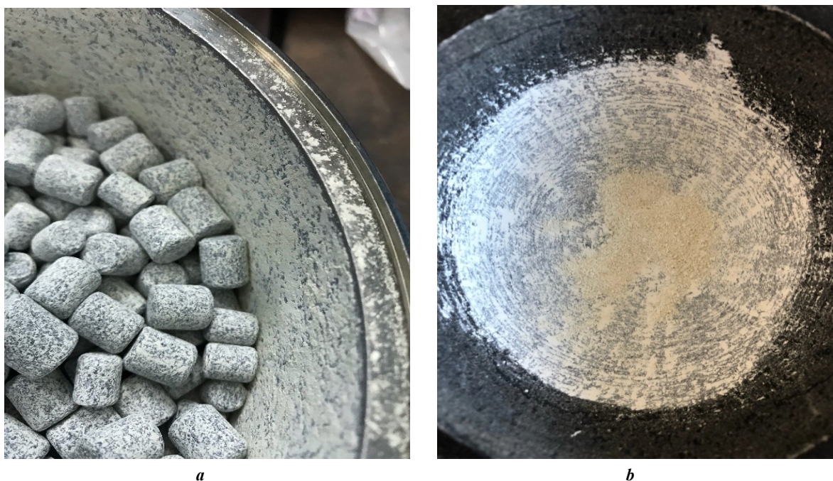
Fig. 3. The appearance of the non-calcined solution combustion (SHS-S) product after grinding: a – in the drum ball mill; b – in the mortar
