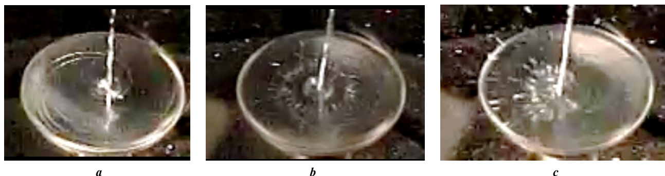
Fig. 6. Changing the distance from the needle to the smooth surface of the bowl: a – 50 mm; b – 100 mm; c – 150 mm
