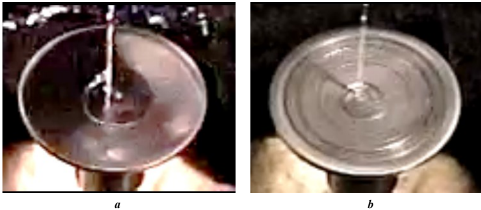
Fig. 3. Changing the surface roughness at a flow rate of 6.69 kg/h and a distance to the bowl of 50 mm: a – a smooth bowl; b – a bowl without treatment
