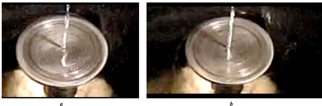
Fig. 5. Changing pressure when liquid is supplied to the surface of the bowl without treatment, needle diameter is 1.5 mm: a – 1 atm.; b – 2 atm.
