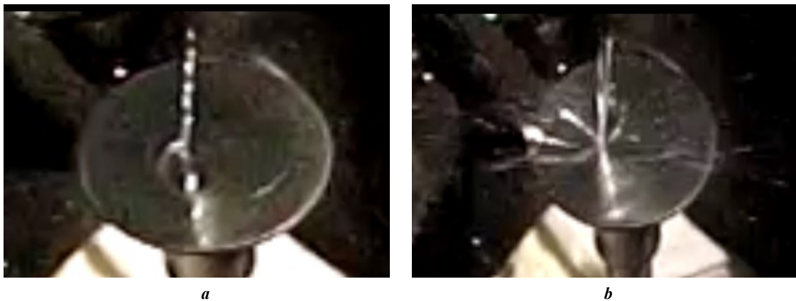
Fig. 10. Changing the pressure of the liquid supplied to the rough bowl surface: a – 1 atm.; b – 2 atm.
