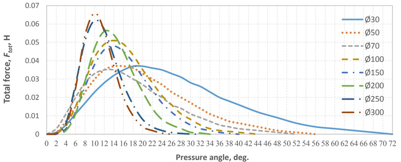
**Fig. 10.** Dependence of the total force acting on a rotating roller with additional powder feed on the pressure angle.
