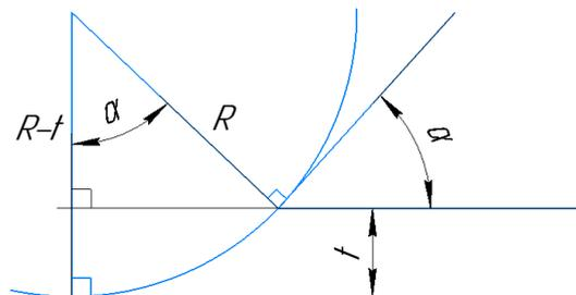
Fig. 6. Scheme for calculating the pressure angle  $\alpha$ .
