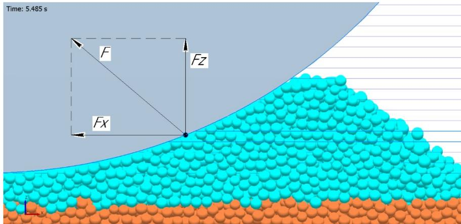
Fig. 5. Calculation of the total force of powder pressure on the roller in each layer
