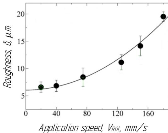
Fig. 4. Dependence of layer roughness on application speed
