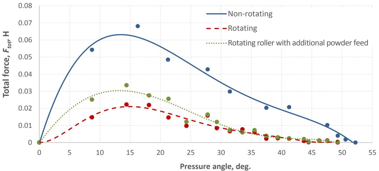
Fig. 11. Dependence of the total force acting on a non-rotating roller and a rotating roller with additional powder feed on the pressure angle. Graphs are given for the roller with a diameter of 50 mm
