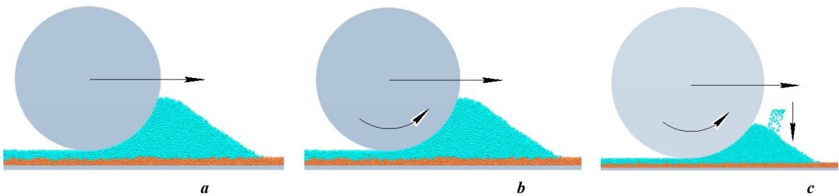
Fig. 3. Ways of applying a powder layer:
