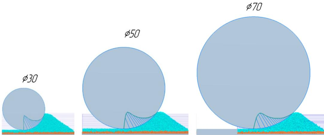
Fig. 9. Force distribution over the rollers with the diameters of 30, 50, 70 mm
