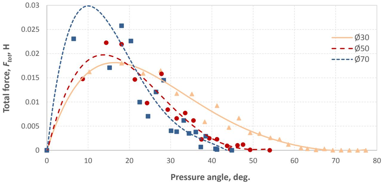
Fig. 8. Dependence of the total force acting on a rotating roller on the pressure angle.
