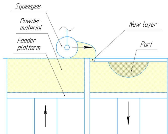
Fig. 1. Basic diagram of the process of applying a powder layer
