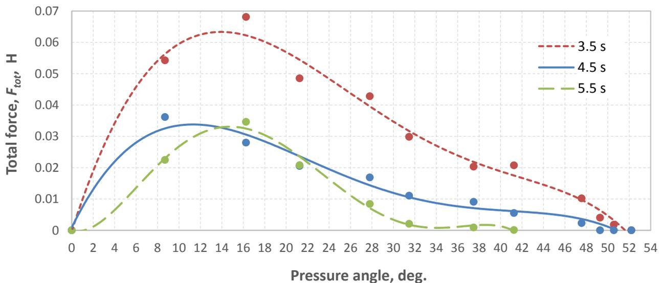
**Fig. 7.** Dependence of the total force acting on a non-rotating roller with a diameter of 50 mm on the pressure angle.
