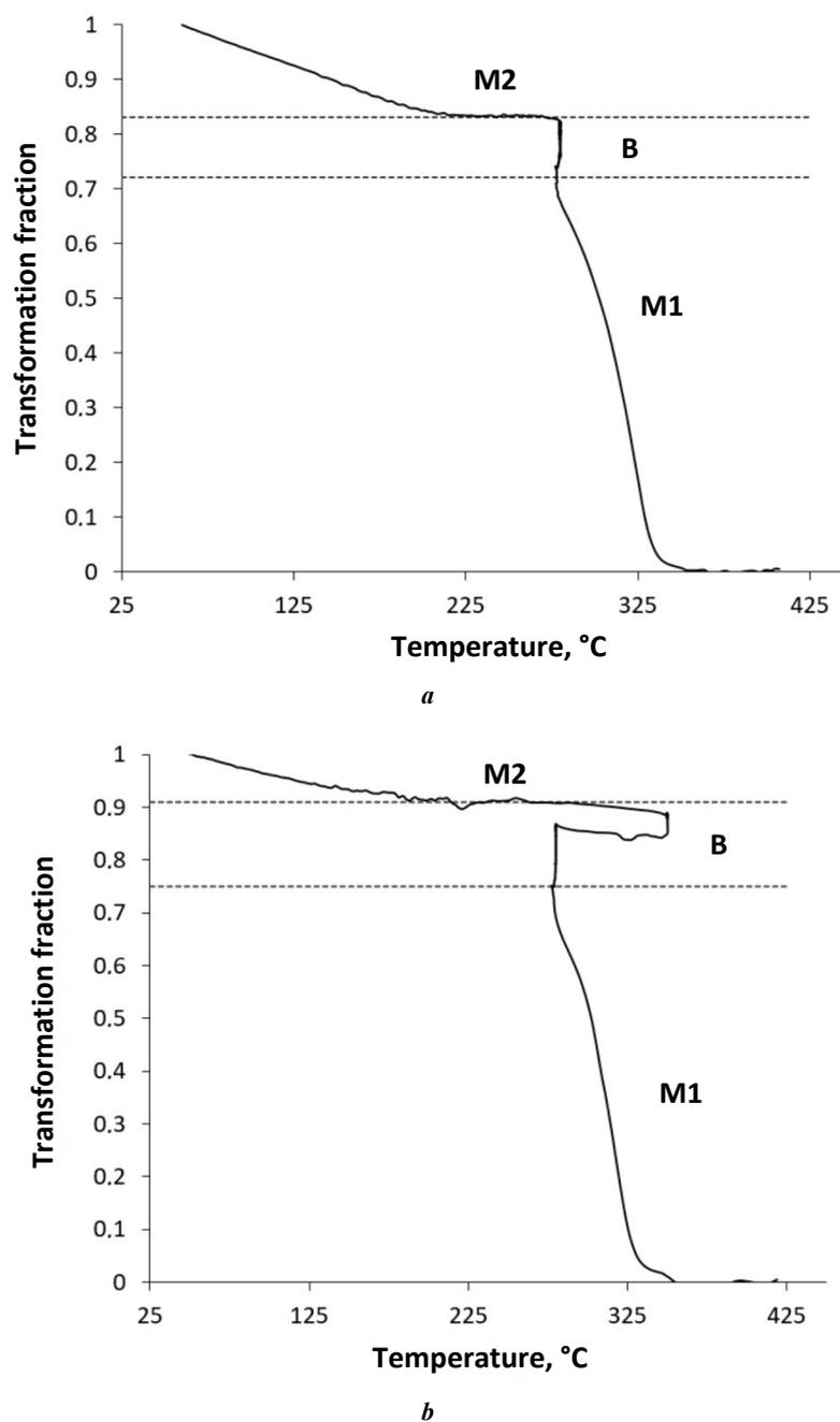
**Fig. 5.** The dependence of the fraction of transformation of supercooled 20Cr2Mn2SiNiMo steel austenite, on the temperature, during step quenching (without taking into account residual austenite): **a** – QP1; **b** – QP2
