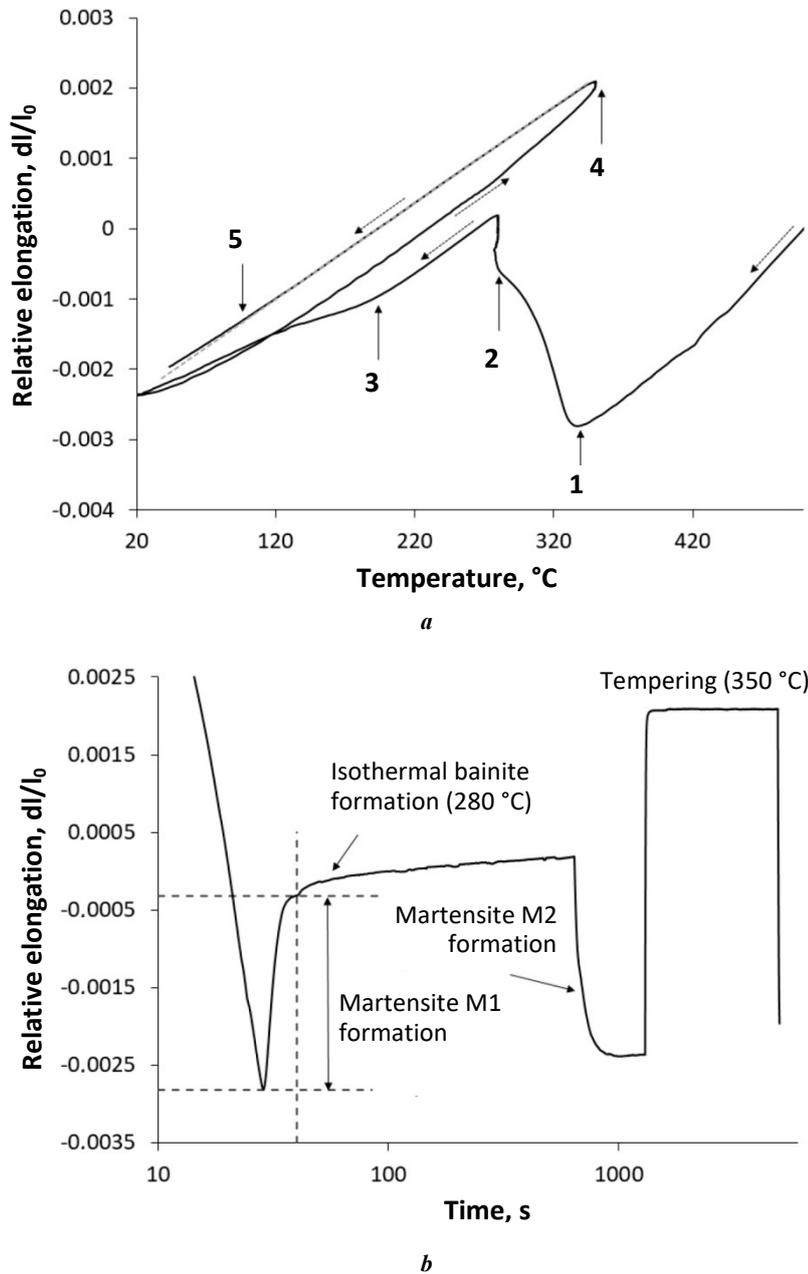
**Fig. 4.** The dependence of relative elongation of the 20Cr2Mn2SiNiMo steel sample on the temperature (a) and time (b) when implementing QPT single-stage quenching with tempering.
