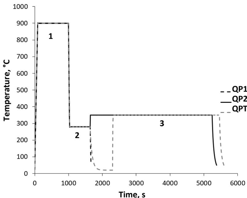
**Fig. 1.** Scheme of implemented modes of step quenching of 20Cr2Mn2SiNiMo steel:
