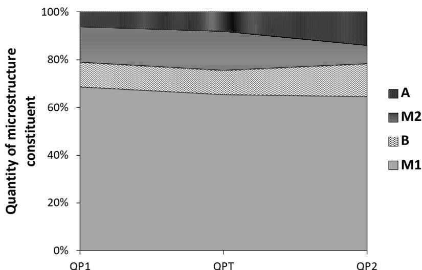
**Fig. 6.** The ratio of the 20Cr2Mn2SiNiMo steel structural components after the implementation of various options of step quenching. M1 – primary martensite; B – bainite; M2 – secondary martensite; A – residual austenite
