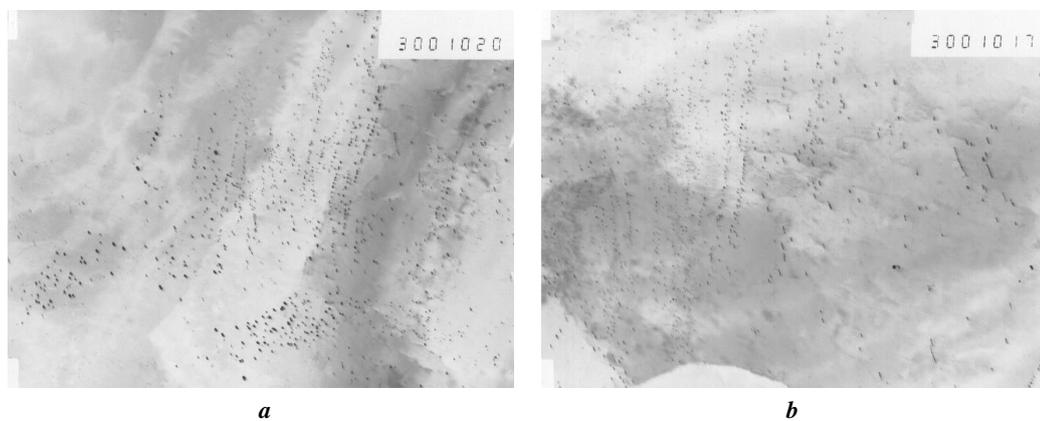
**Fig. 4.** Nanosize particles of carbonitrides in the steel 1:
