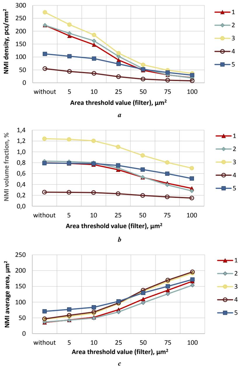
**Fig. 1.** Statistical parameters of NMIs of the steels under study at different filtration levels:
