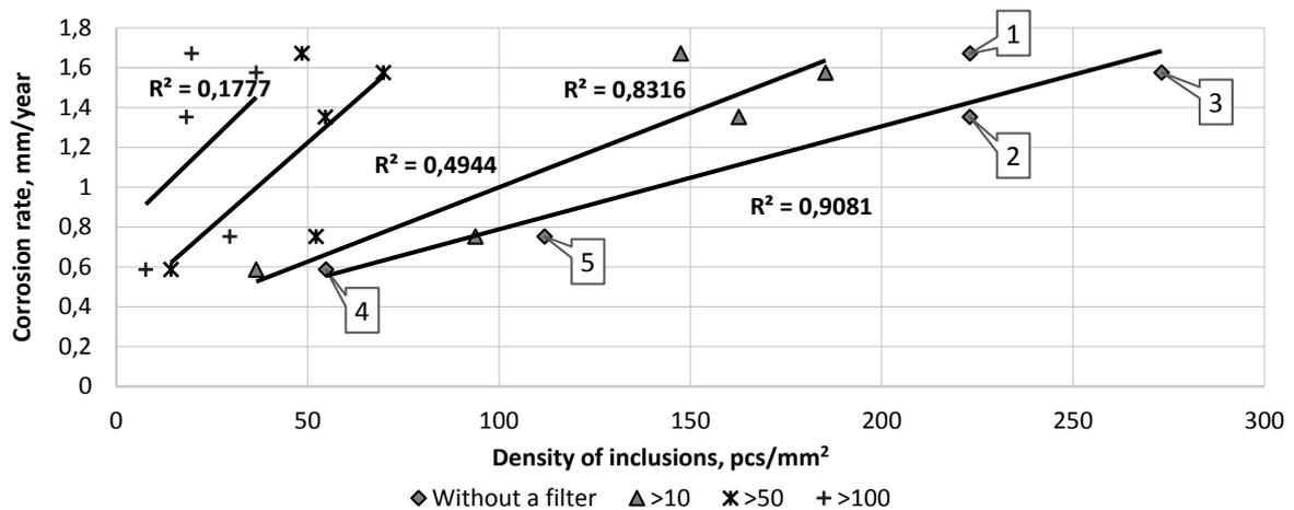
**Fig. 2.** Correlation of NMI density and corrosion rate in the steels under study when varying the inclusion filtration level (by their area)
