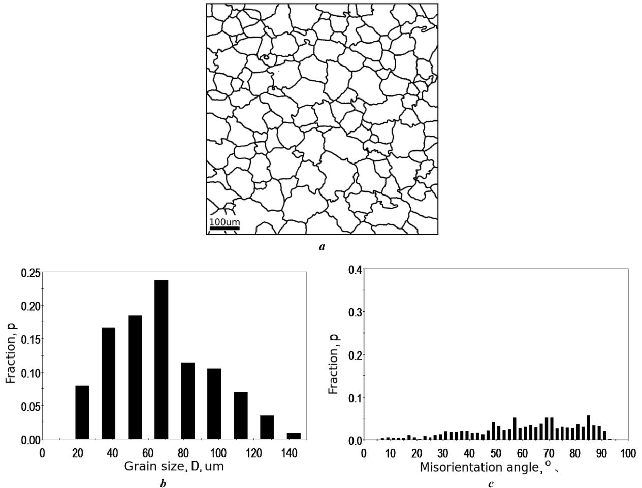
**Fig. 1.** The initial structure of the MA14 alloy (a), histograms of the grain size distribution (b) and the crystal lattice misorientation at the grain boundaries (c)
