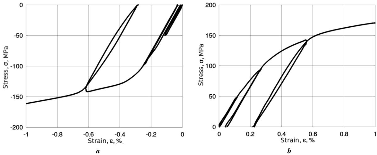
**Fig. 2.** Loading – unloading diagrams of the MA14 alloy.
