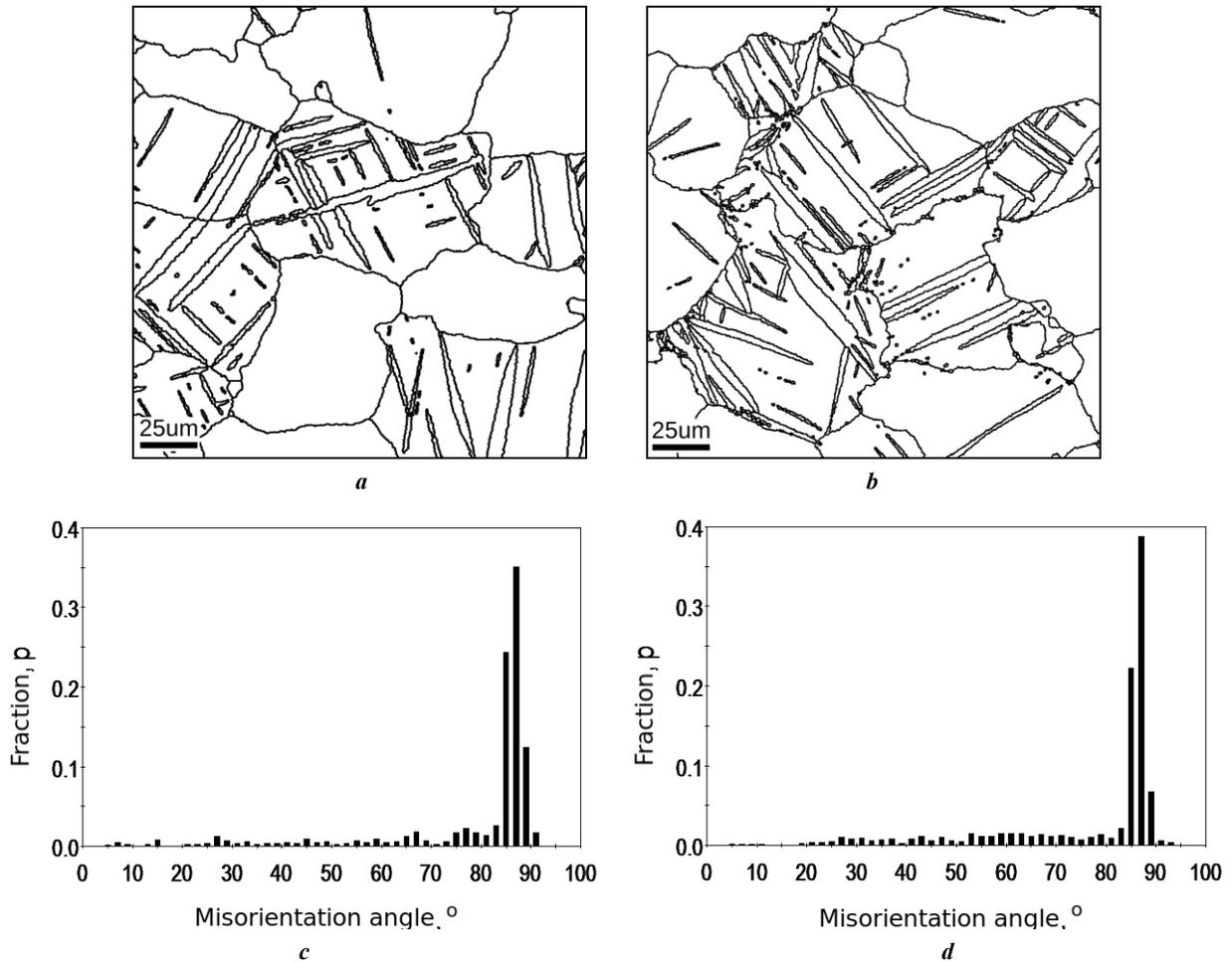
**Fig. 5.** MA14 alloy structure after compression (a) and tensile (b) tests, histograms of the crystal lattice misorientation angles at the grain boundaries after compression (c) and tensile (d) tests
