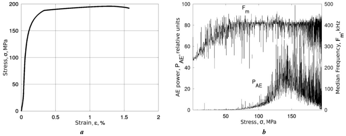
**Fig. 4.** Loading diagram of the MA14 alloy sample (a) and acoustic emission parameters depending on the stress (b)
