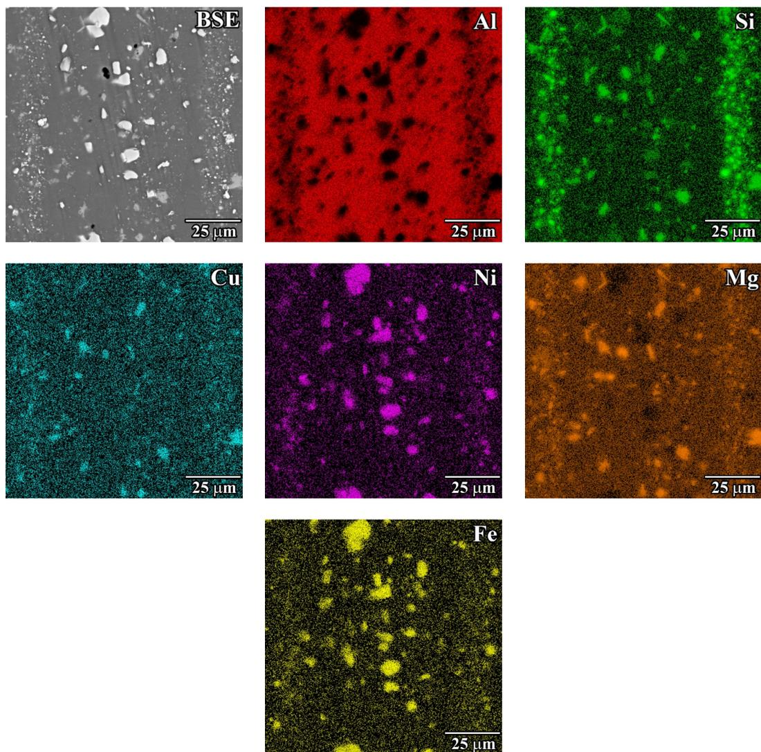
*Fig. 5. Distribution maps of the primary alloying elements in the center part of the polished stir zone surface. EDS analysis*
