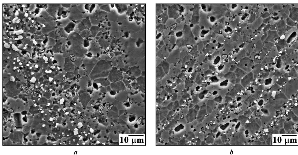
*Fig. 6. Typical grain microstructure in the center (a) and on the periphery (b) of the stir zone. SE mode SEM images*
