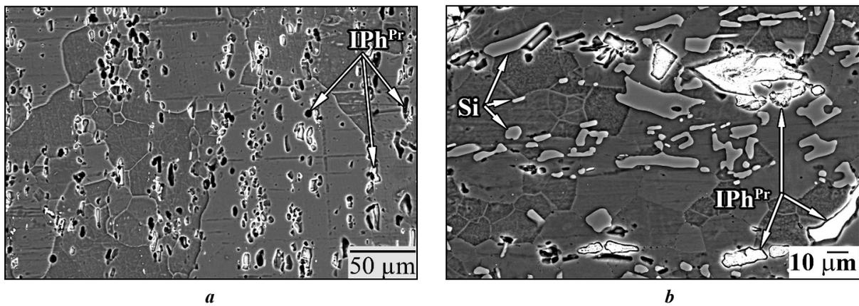
Fig. 1. Typical microstructure of the AK4-1 (a) and AK12D (b) alloys in the initial heat-treated state.  $IPh^{Pr}$  – primary intermetallic phases, Si – silicon particles. BSE mode SEM images
