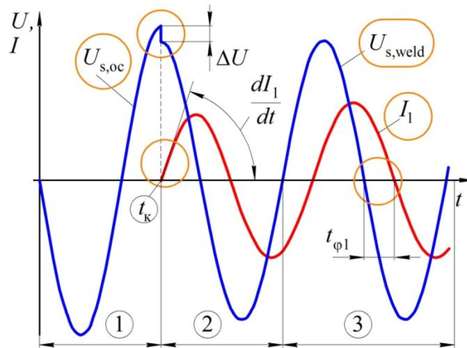
**Fig. 2.** Current and voltage oscillograms at full-phase switching-on.
