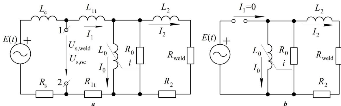
**Fig. 3.** Calculated equivalent circuit of the contact welding machine with on (a) and off (b) thyristor contactor
