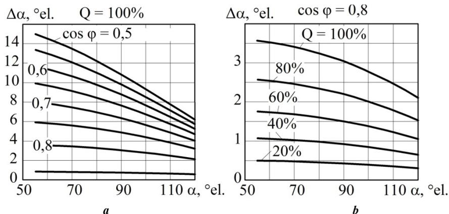
Fig. 5. The dependence of the allowance  $\Delta\alpha$  on the control angle  $\alpha$  at different loads by power  $Q$  for  $\cos\varphi=0.8$  (a) and at 100 % load of the welding machine (b)
