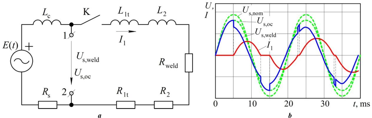
**Fig. 1.** A simplified electric equivalent circuit of the contact welding machine when connecting to a non-ideal circuit (a) and oscillograms of the current and voltage (b).  $E(t)$  – ideal sinusoidal voltage source;
