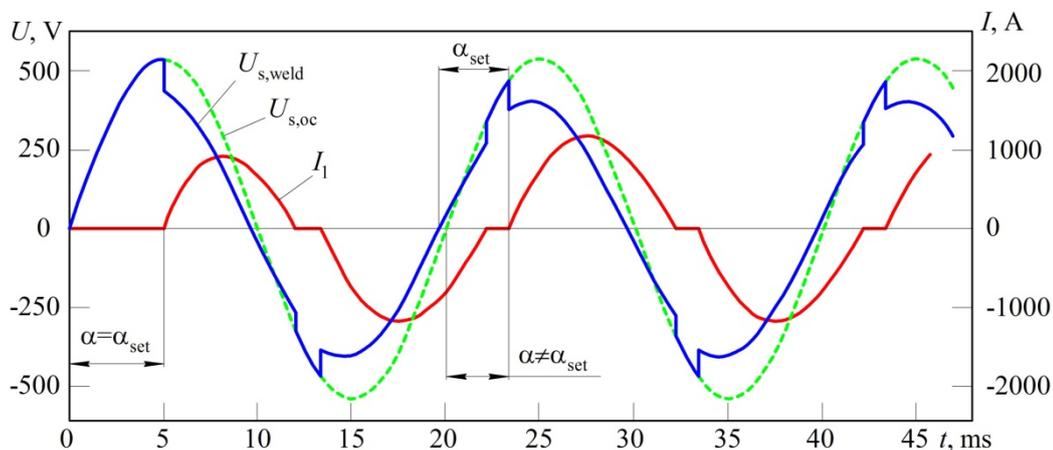
Fig. 4. Calculated voltage and current curves built taking into account the supply mains parasitic parameters
