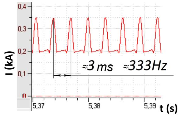
**Fig. 2.** External appearance of the oscillogram of the modulated current of the Lorch S8 Pulse XT power supply
