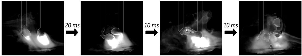
**Fig. 8.** Cross-movement of electrode drops with drop transfer disruption ( $I=350\text{ A}$ ;  $U_{arc}=30\text{ V}$ )
