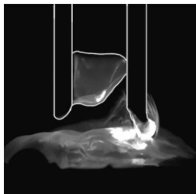
**Fig. 4.** Displacement of the common drop to the upper part of the arc reaction zone
