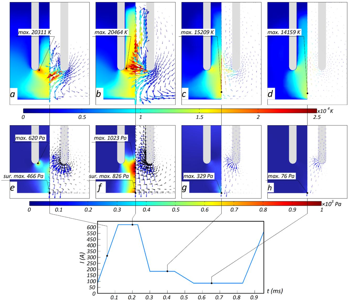
**Fig. 9.** Distribution of temperature in the model arc, direction and plasma flow rate (a–d);
