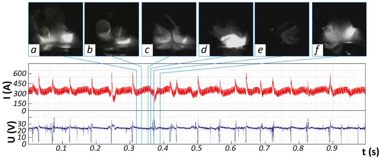
**Fig. 3.** External appearance of the oscillogram of the direct current and voltage and high-speed video footage ( $I=280\text{ A}$ ;  $U_{arc}=23\text{ V}$ )
