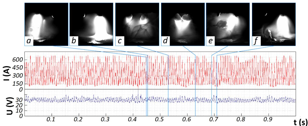
**Fig. 7.** External appearance of the oscillogram of the pulse current and voltage and high-speed video footage ( $I=280$  A;  $U_{arc}=30$  V)
