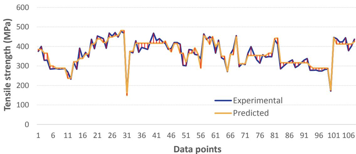
**Fig. 9.** Experimental vs predicted values of tensile strength (ANN)
