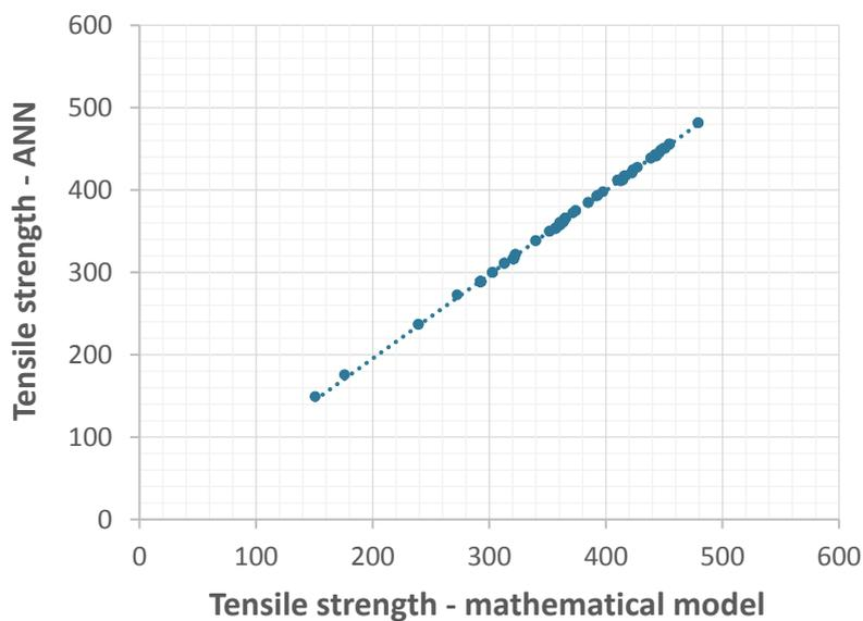
**Fig. 8.** Tensile strength predicted using ANN vs mathematical model
