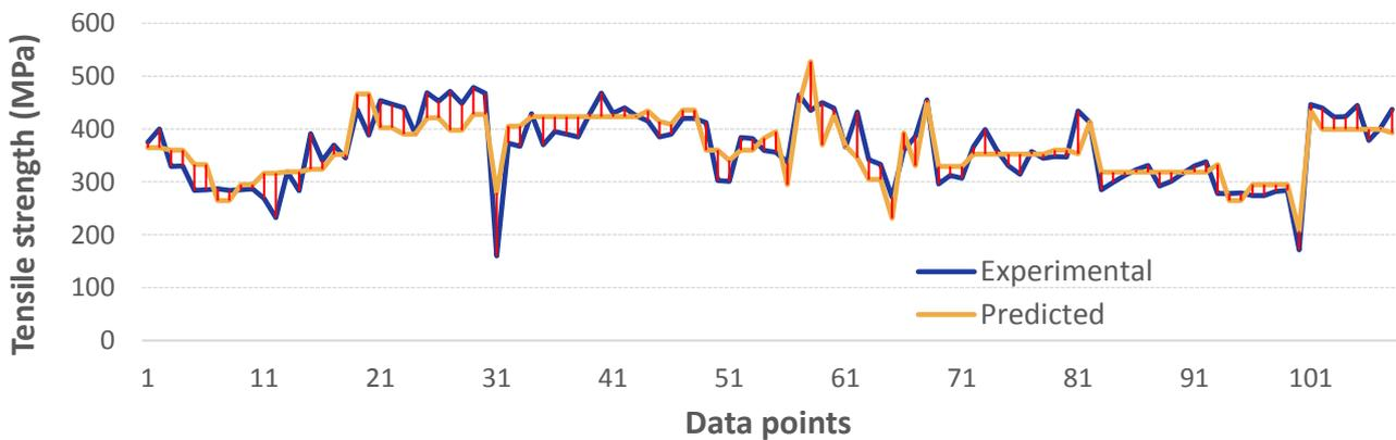
**Fig. 11.** Experimental vs predicted values of tensile strength (polynomial regression)
