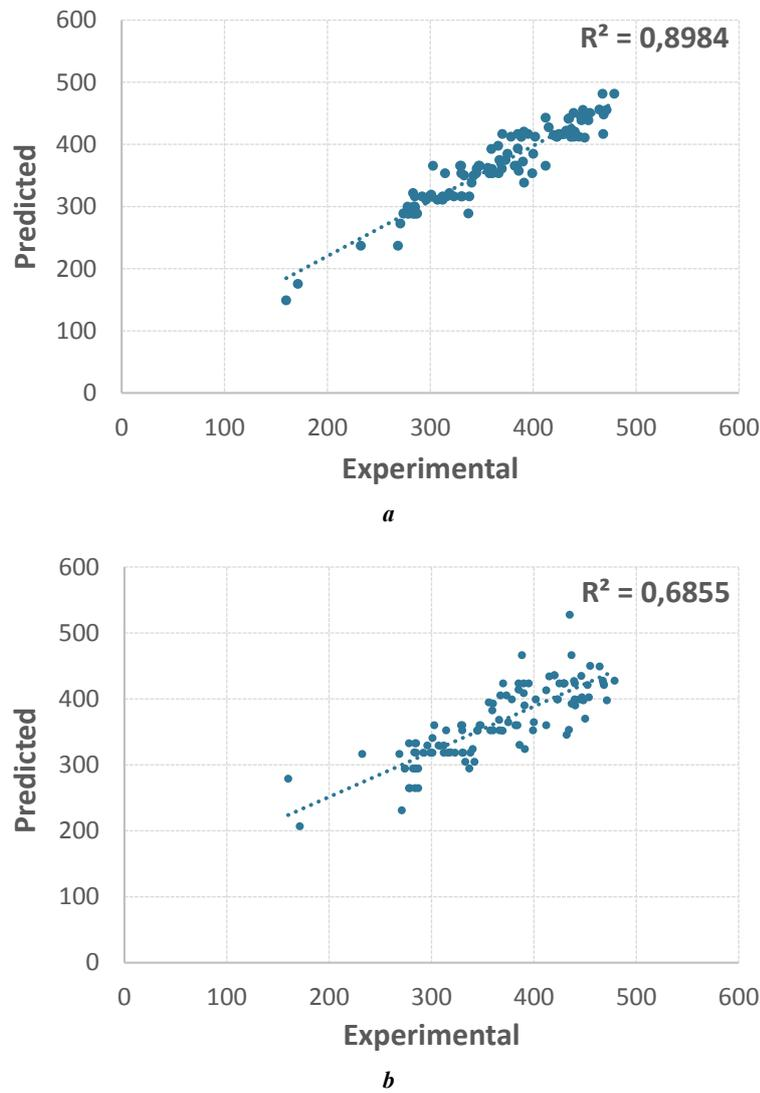
**Fig. 10.** Comparison of the measured vs predicted tensile strength:
