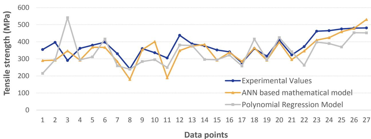
**Fig. 12.** Experimental vs predicted values of tensile strength for new data points
