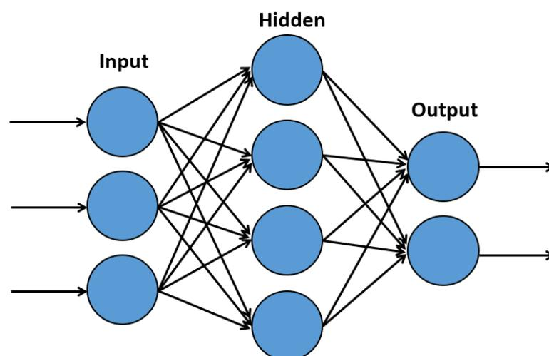
**Fig. 1.** Architecture of an artificial neural network
